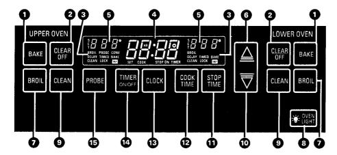
NOTE: Oven has controls for upper oven and lower oven. Be sure to set the correct control. Pads on the left side of panel are for the upper oven. Pads on the right side of panel are for the lower oven. The TIMER ON/OFF, COOK TIME, and STOP TIME pads can be used for either oven.
